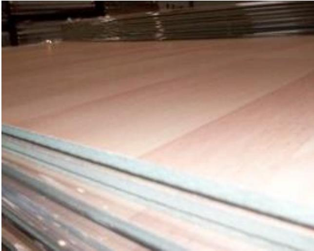
Figure 3: Finished product (Melamine faced MDF boards)
