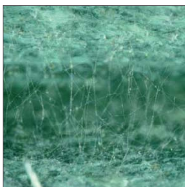
Fig. 7: Mould on test specimen 59 (H40), 40-fold enlargement.
